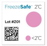
**Example:** The 2°C threshold indicator dot will be as dark as the reference dot in 90 minutes at 1°C (within 1 year of date of manufacture). If exposed to 1°C for some period of time, say 60 minutes, the indicator dot will appear darker than prior to use and lighter than the reference dot.
