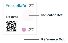
An indicator dot may start clear, or light magenta, and show color darkening but remain lighter than the reference dot. This means the indicator saw exposure to the threshold temperature for less than the specified activation time.
